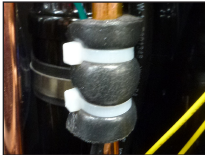
Figure 8: Thermistor attached to the refrigerant line.
